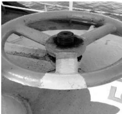
**Gambar 20.** *Tank Cleaning Valve*
